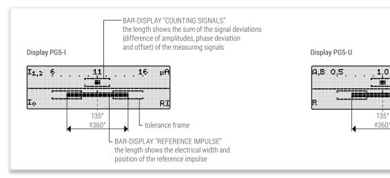
**PG5-I** for linear encoders with square-wave output signals **PG5-U** for linear encoders with sinuoidal voltage signals 1 Vpp
